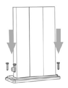
Fissaggio a terra Fastening to ground
