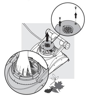
If you notice debris trapped in the impeller, open the impeller and remove the debris.
