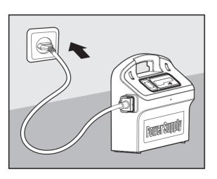
Plug in the power supply and leave it in the OFF position.
