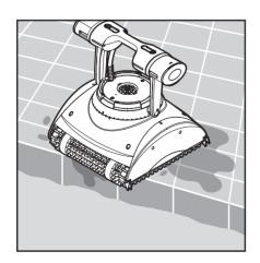
Place the Pool Cleaner on the edge of the pool and let the water drain out.
