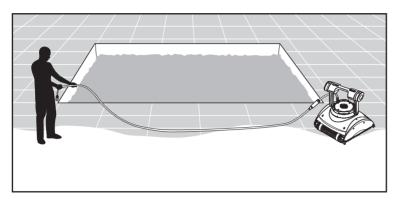
Unwind the cable and stretch it out completely so that it has no kinks.
