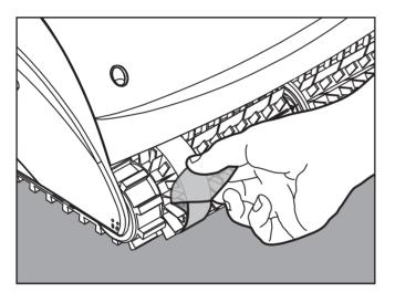
While pushing in the handle buttons turn the ring so that the large projection on the ring lines up with the projection on the Pool Cleaner body.
