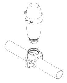
Seal the hose clamp with the cap provided in the **Blue Fit50** box.
