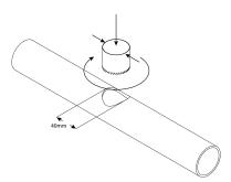
Place both parts of the hose clamp on each side of the pipe so that the holes coincide, and screw the hose clamp.
